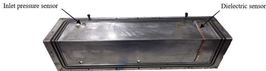
Figure 1. Integration of pressure transducers and dielectric sensors on an L-Shape Mould.
