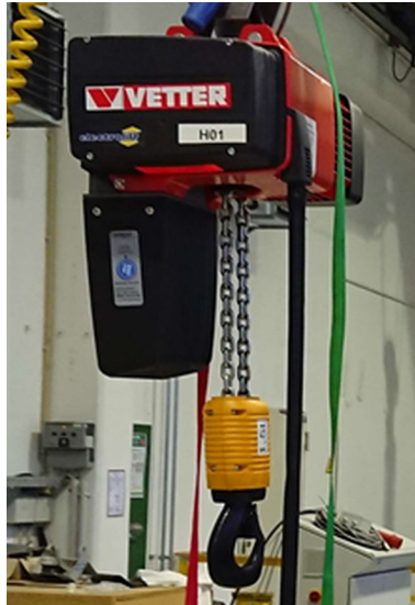
Fig. 3. Chain hoist with 2/1 reeving system.
