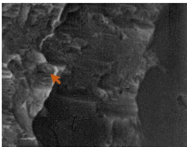
Fig. 20. Structure of a cement stone made of blast-furnace cement with a ferromagnetic additive (BFC+FA). Phase-contrast mode. The arrow marks an ingrown dust particle.
