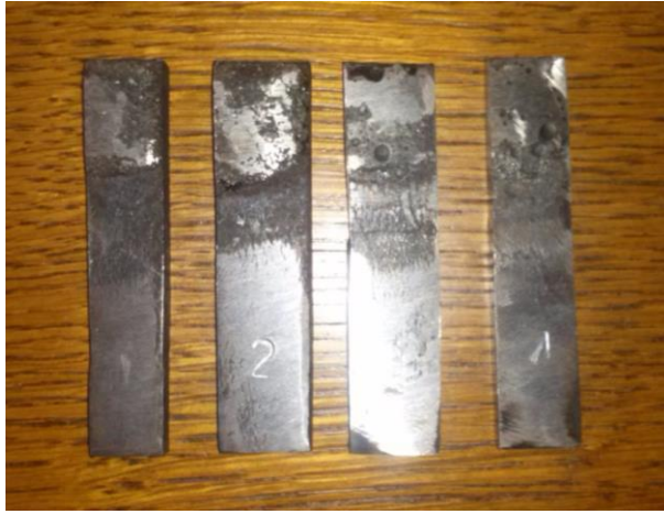
Fig. 4. Samples of the cutters' hardsurfacing overlays, prepared for X-ray phase analysis
