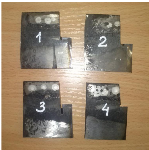
Fig. 3. Samples of the cutters' hardsurfacing overlays, prepared for emission spectral analysis
