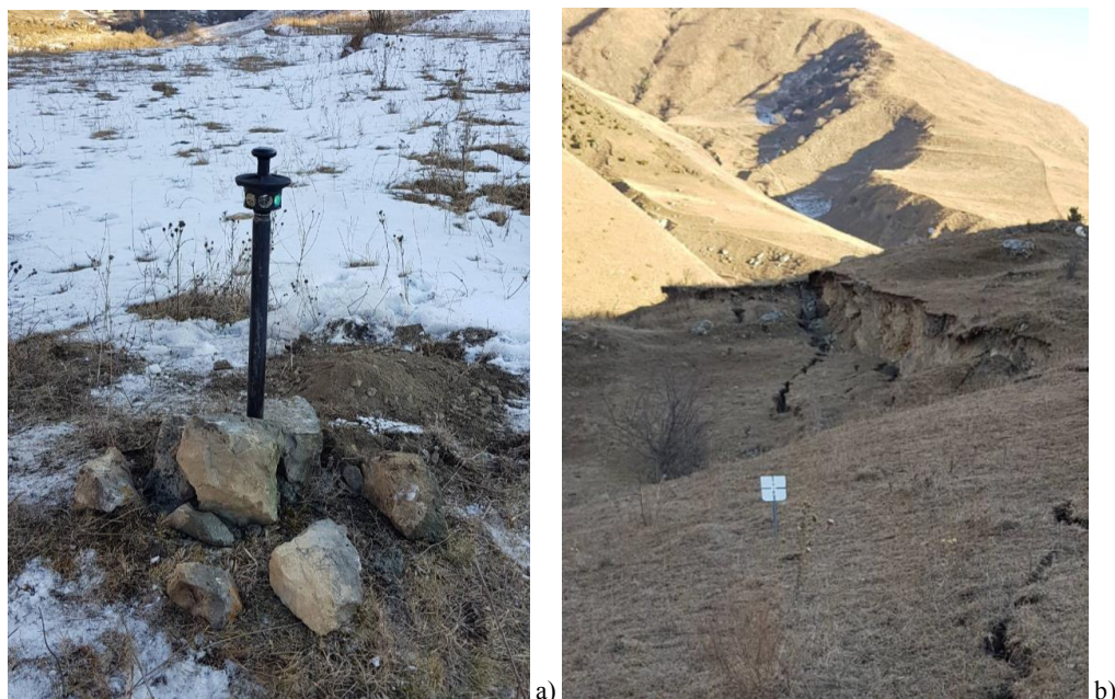
Fig. 6. Arrangement of the reference point with a prism installed at the time of measurements (a) and a reference point - reflector (b)
