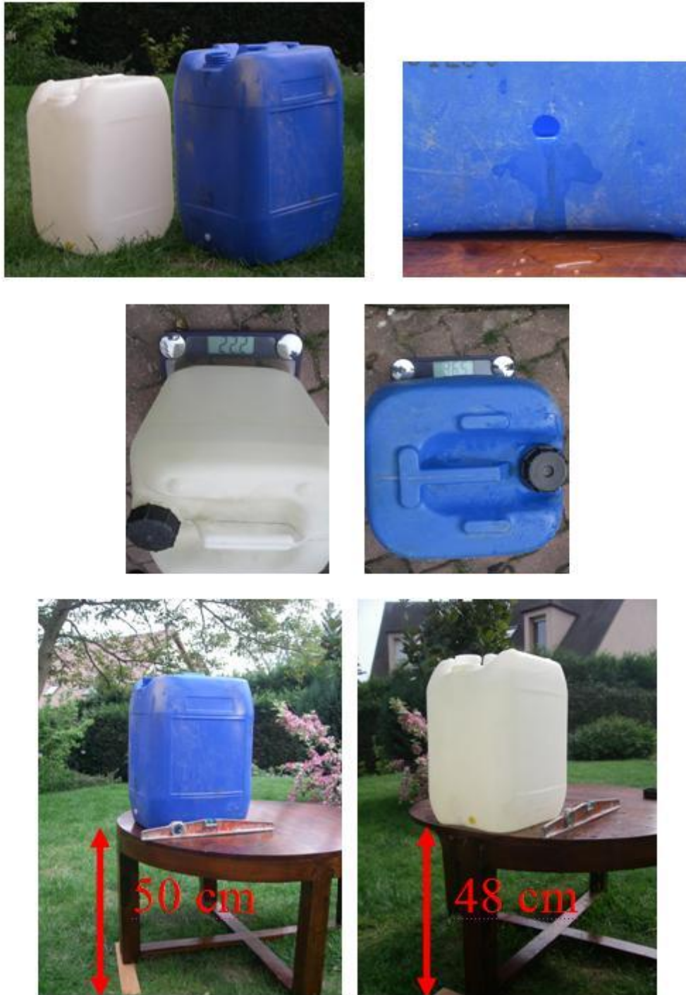
Figure 1: Example of atypical experiments in fluid mechanics: emptying jerry cans, preparation of experiments.
