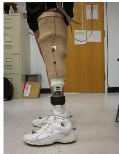
Figure 50: Subject TT01 on Diagnostic socket instrumented with ZEBRA socket pressure sensors and with an iPECS unit distal to the socket
