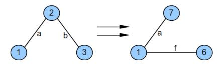
**Figure 3:** Example of a rule. Shown are the left-hand side and the right-hand side. Note how the rule changes vertex labels, edge labels, and the edge structure.
