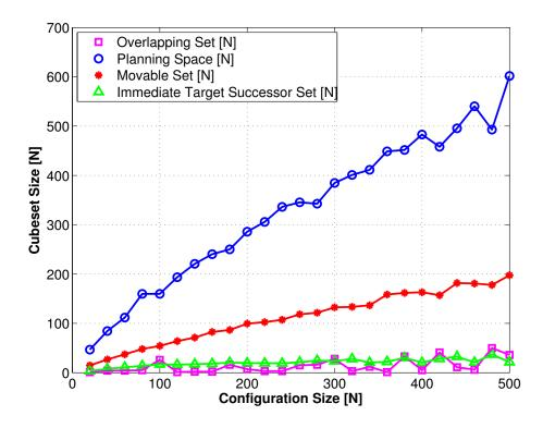
**Figure 28:** Cubeset sizes break down for reconfigurations of size 20 to 500. Shown are average values for each reconfiguration size.
