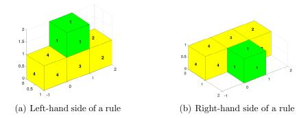
Figure 13: Visual representation of a rule that shows a convex motion of cube 1.
