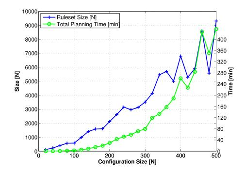
**Figure 23:** Ruleset size and total planning time for reconfigurations of sizes 20 to 500
