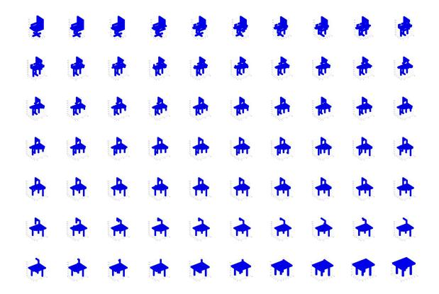
**Figure 15:** Reconfiguration sequence from a chair configuration to a table configuration in free space
