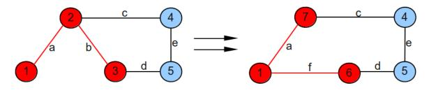
**Figure 4:** Example of a rule application. The subgraph matching the left-hand side of the rule shown in Fig. 3 is highlighted.
