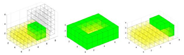
(a) Initial (transparent) and tar- (b) Movable nodes (opaque) as (c) Immediate target successor poget (transparent) configuration and part of the initial configuration sitions (opaque) as neighboring pooverlapping nodes (opaque) (transparent) sitions of the initial configuration (transparent)
