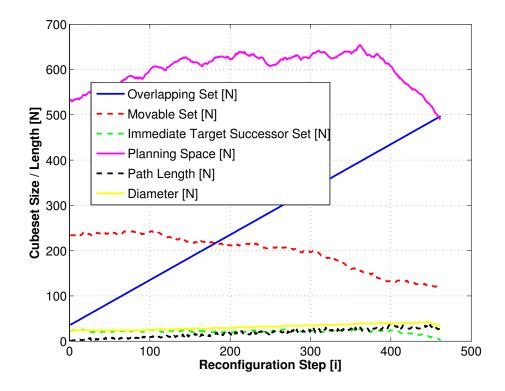
**Figure 27:** Cubeset sizes break down for a single reconfiguration of size 500 requiring 462 paths to be planned.
