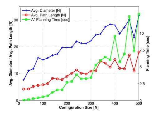
**Figure 25:** Average diameter, path length, and planning time for reconfigurations of sizes 20 to 500
