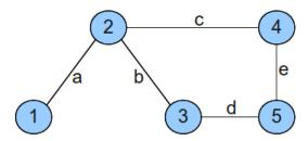
**Figure 1:** Example of a labeled graph. Vertex labels are represented by integers, edge labels by letters.
