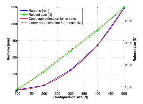
**Figure 21:** Number of generated rules and required runtime for ruleset generation of box configurations
