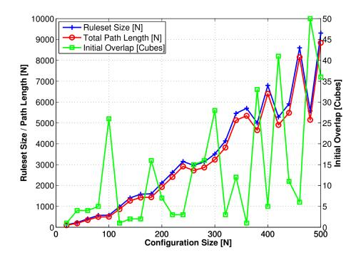
**Figure 24:** Ruleset size and total path length for configurations of sizes 20 to 500. The initial overlap of the initial and target configuration is shown in green.
