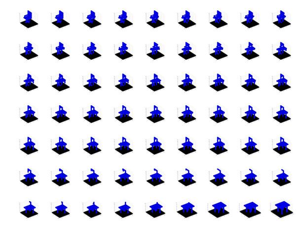
**Figure 19:** Reconfiguration sequence from a chair configuration to a table configuration in obstacle-constrained space. Obstacles are shown in black.
