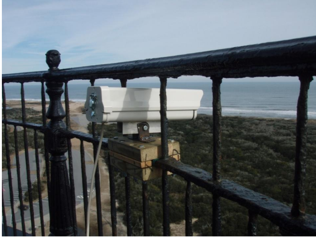
Figure 5: Camera securely attached to the railing of the Cape Hatteras Lighthouse using a custom fabricated mount.
