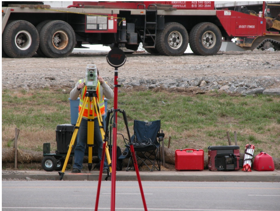
Figure 30: Initial reading of reference target taken to orient the total station
