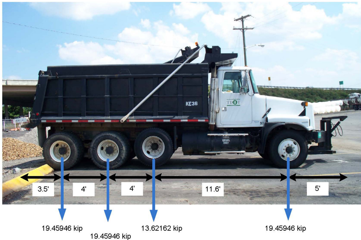
Figure 79: Force distribution of truck used during live load testing
