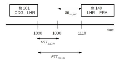
Figure 7: Incorporating Scheduling Buffers to Increase Robustness
