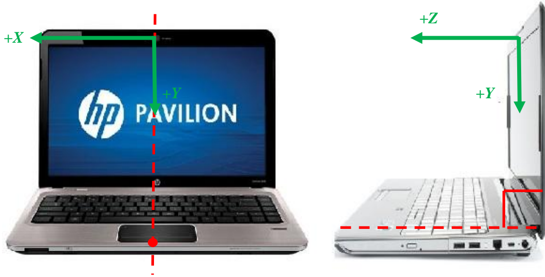
Figure 8: (a) Dotted line is line with camera center, the red dot indicates a reference point of measurement during the experiment. (b) Profile of the laptop. The screen orientation was kept perpendicular to the horizontal at all times. Camera axes and laptop translation axes are in the same direction. [40].
