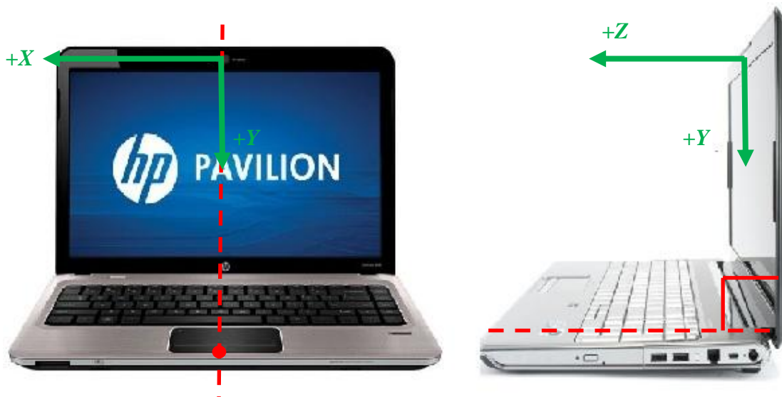
Figure 19: (a) Dotted line is line with camera center, the red dot indicates a reference point of measurement during the experiment. (b) Profile of the laptop. The screen orientation was kept perpendicular to the horizontal at all times. Camera axes and laptop translation axes are in the same direction [37].
