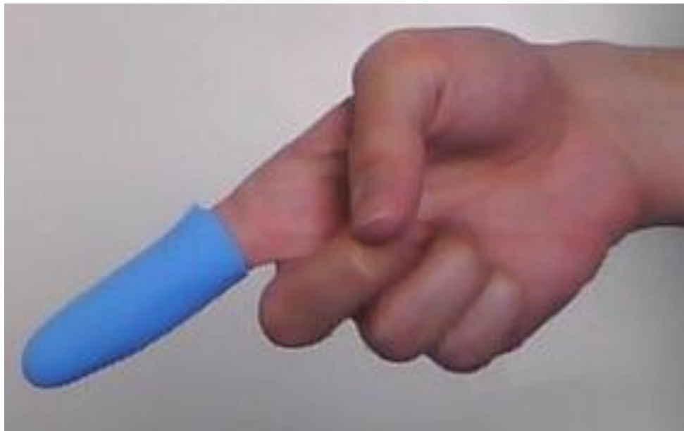
Figure 13: Finger glove used for finger gesturing experiment. The finger glove was cut from a Clorox cleaning glove purchased at a Target store.
