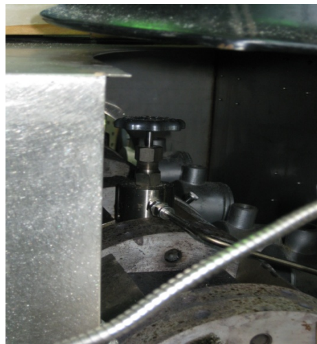
Figure 3.3: N_2 supply to the extruder just below the valve
