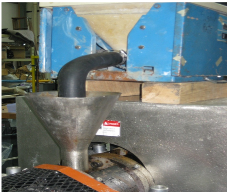
Figure 3.5: Closed screw feeder from covered hopper, black transfer hose and extruder hopper
