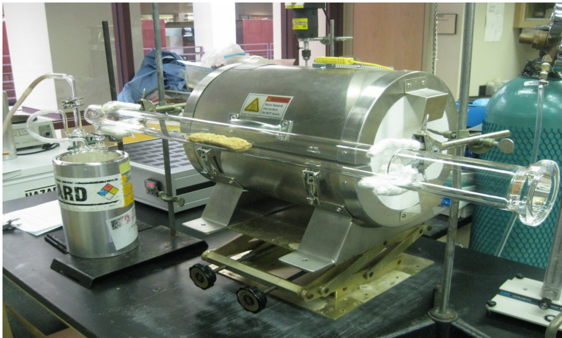
Figure 4.1: Tubular pyrolysis reactor consisting of wood sample, pyrolysis tube, condenser and heater
