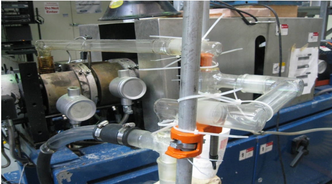
Figure 3.4: Condenser to collect volatile gases using liquid nitrogen as coolant
