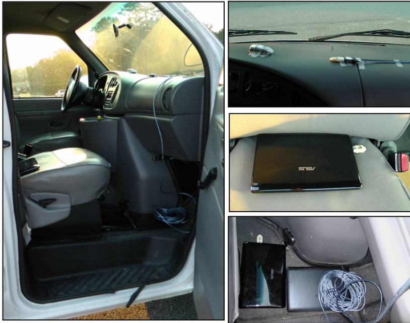
Figure 57: Probe Vehicle Bluetooth Adapter & GPS Configuration
