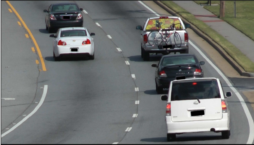
Figure 12: Ideal Camera View for Arterial Roadway License Plate Captures
