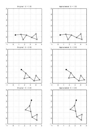
Fig. 3. Comparison of agent motion between original dynamics Eq. (5) (left) and rigid-link approximated dynamics Eq. (18) (right). The filled circle in each figure is the leader agent.
