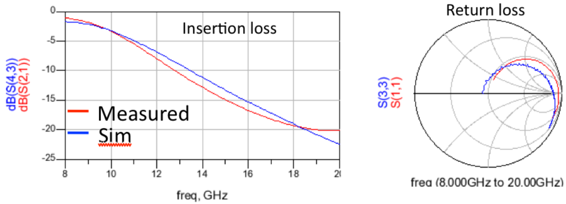
Figure 28. Simulated and measured comparison of matching network in PA
