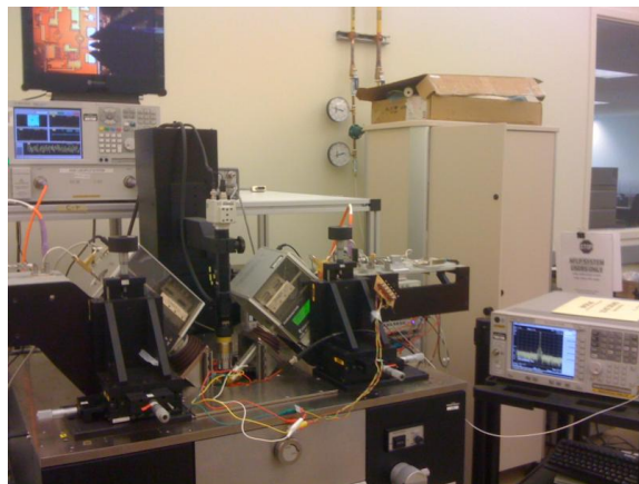
Figure 21. Photograph of TX measurement setup. Spectrum analyzer is shown with output signal from PA. [Dr. John Cressler's Group, Georgia Tech Equipment]
