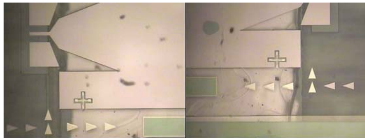
Figure IV.13 - Alignment result of bonding the top and bottom sapphire substrate layers (both layers have metallized alignment marks on the bonding side).
