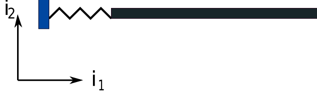
Figure 7: Schematic of a beam restrained by longitudinal spring attached to its root
