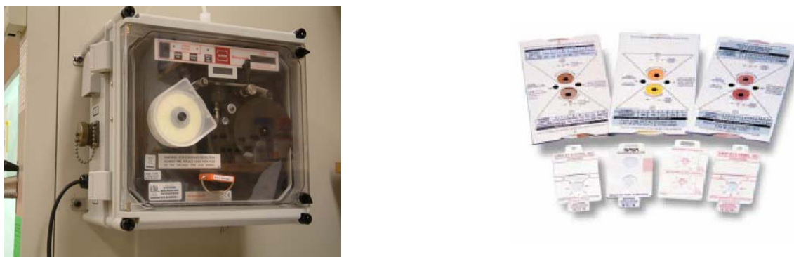
Figure 2.34 ChemCassette hydrazine monitoring system and hydrazine monitoring badges
