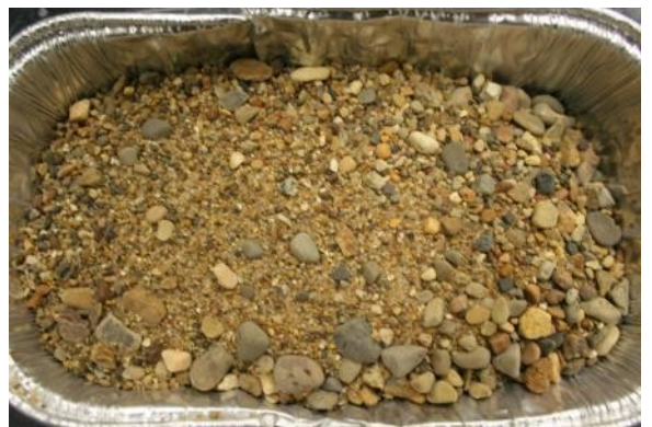
(f) Galena road gravel
