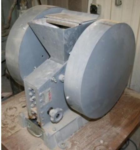
Figure 3.3. Jaw crusher used for crushing aggregates.
