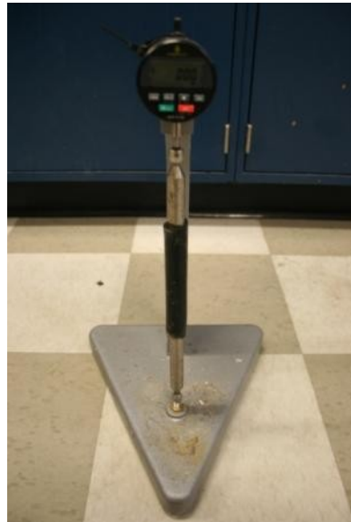
Figure 3.5. Comparator for expansion measurements.
