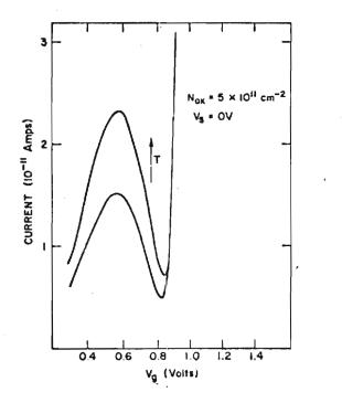
Fig. 2.7 The experimental results of Hartstein and Fowler for the channel conductivity of a MOS field effect transition. Note the peak in the conductivity below the onset of metallic conduction indicating the formation of an impurity band. semiconductor inversion layer.
