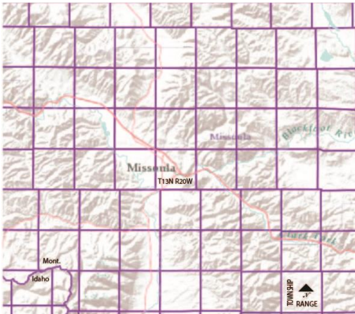
Figure 27: An example of the PLSS Township-Range vector layer from the Montana GIS Clearinghouse.
