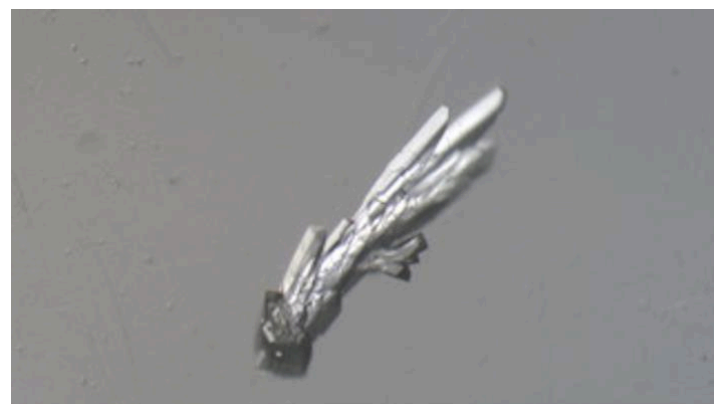
Figure 5. Crystallization using microbatch under oil for Hex AA
