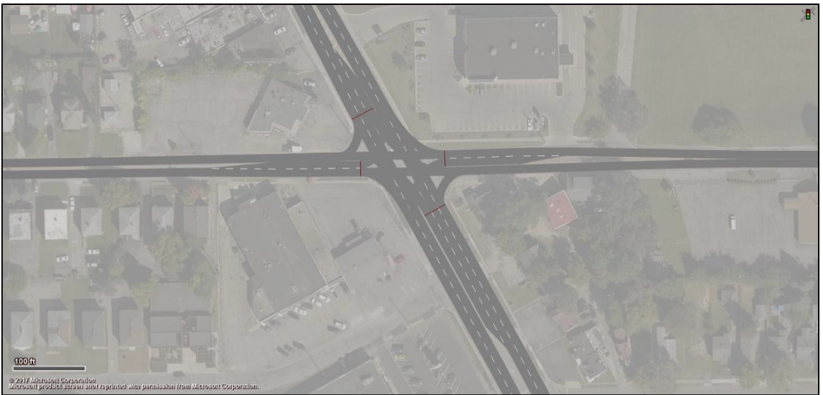
Figure C-4 Intersection Layout (Links and Connectors) in PTV Vissim
