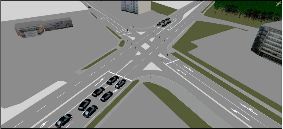
Figure C-7 Intersection (3D Model) in PTV Vissim
