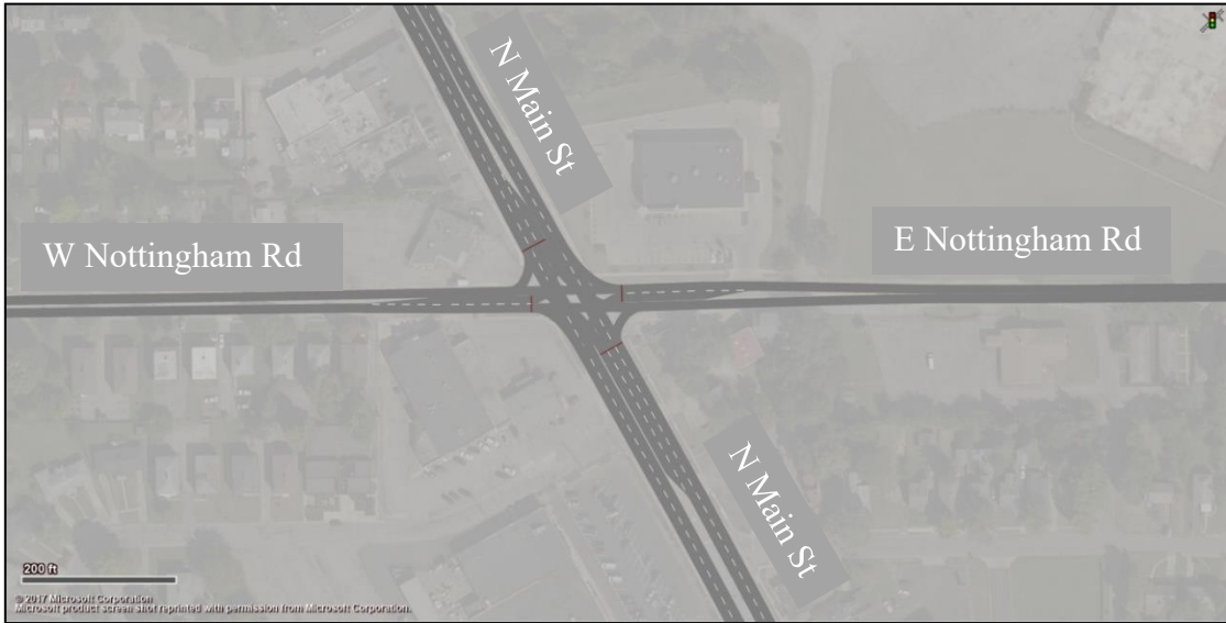
Figure 3.11 Intersection Layout in PTV Vissim Using Links and Connectors
