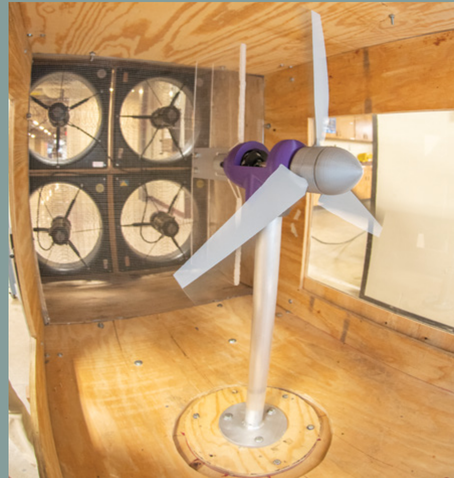
A small wind tunnel in Engineering Hall provides a place for students and researchers to test their wind turbine designs.
