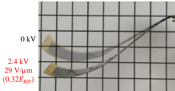
Figure 3.6 Unimorph actuator bending due to the DEA (with the 90 \mu\text{m} elastomer) actuation on a 5 mm grid background.
