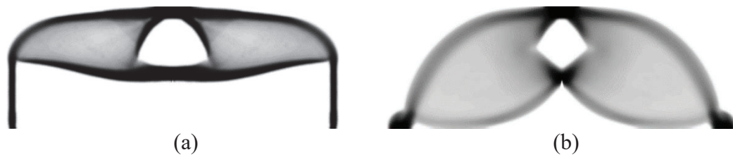
Figure 5.12. Optimized (a) stress-constrained and (b) compliance-based designs.
