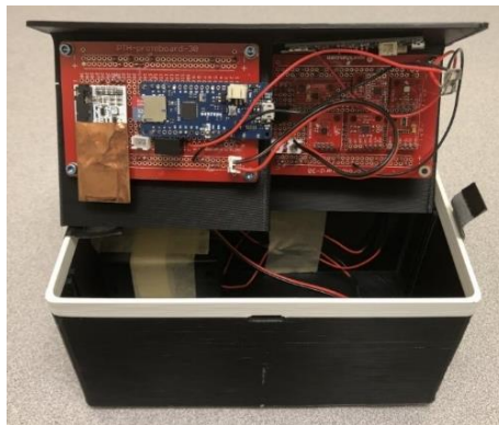
Figure 49: Modified avionics payload flown onboard parabolic Zero-G flight
