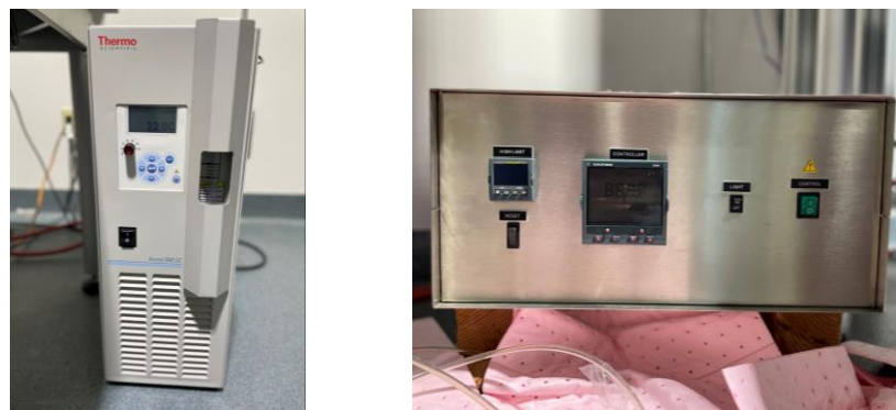
Figure 6.2 Chiller and temperature controller
