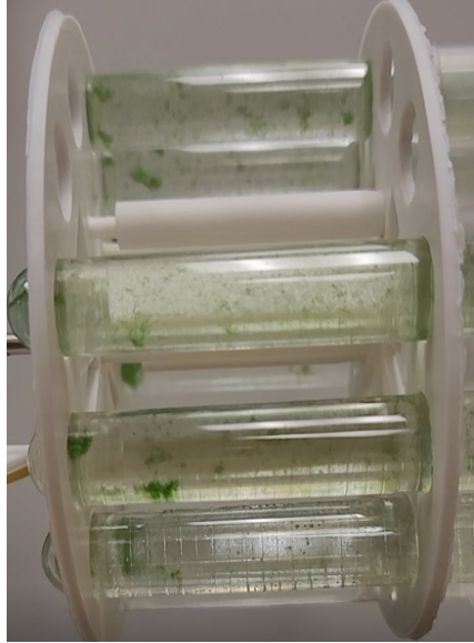
Figure 4.16 Experimental demonstration with 8 RPM rotation on the clinostat using A. platensis .
