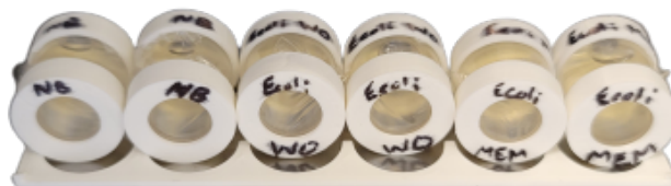
Figure 3.6 Prototype vessel in three groups: only media, with gas-exchange membranes and without gas exchange membranes.
