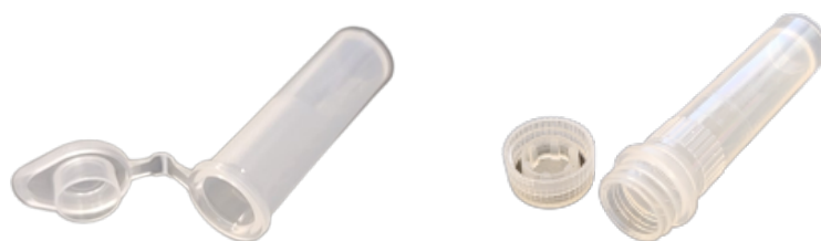
Figure 3.5 The flip cap tube (left) and the screw cap (right) used during experiments.
