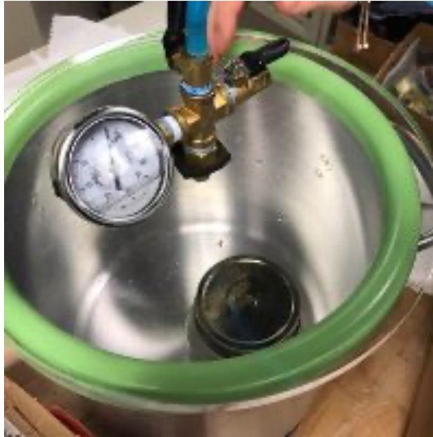
Figure 36: Shown above is a laboratory experiment of low-pressure vaporization.
