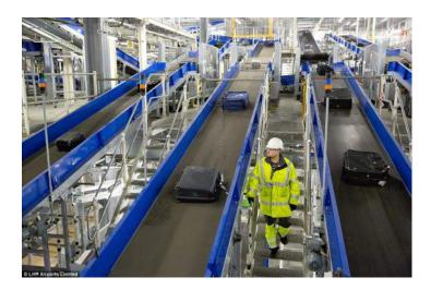
*Figure 2*. Heathrow Terminal 5 baggage handling system. Adapted from "Ever wondered what happens to your bag at an airport? Behind the scenes on the luggage conveyor belts of Heathrow Terminal 5", by Duell, 2014. Retrieved from http://www.dailymail.co.uk/ news/. Copyright 2014 by Duell.
