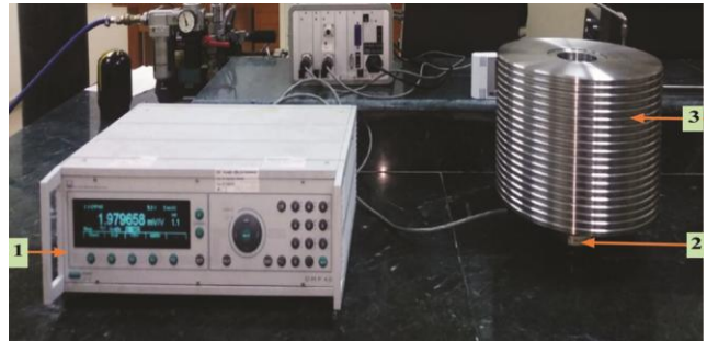
Fig. 1 — Shows method 1 calibration mechanism: 1. DMP40, 2. Load cell, 3. Deadweights
