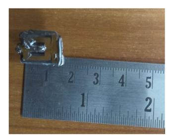
Fig.6 — Fabricated absorber loaded slotted PIFA antenna
