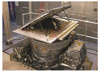
Fig. 34 — Photo of the Mini-SAR antenna during testing<sup>4</sup>.
