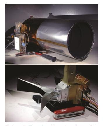
Fig. 3 — The Photographs of Lunar Reconnaissance Orbiter Camera [(a) Wide angle camera(WAC) and (b) Narrow Angle camera (NAC)]<sup>8</sup>.
