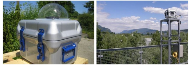
FIGURE 3 Fisheye lens camera and its installation at Sorea's site in France
