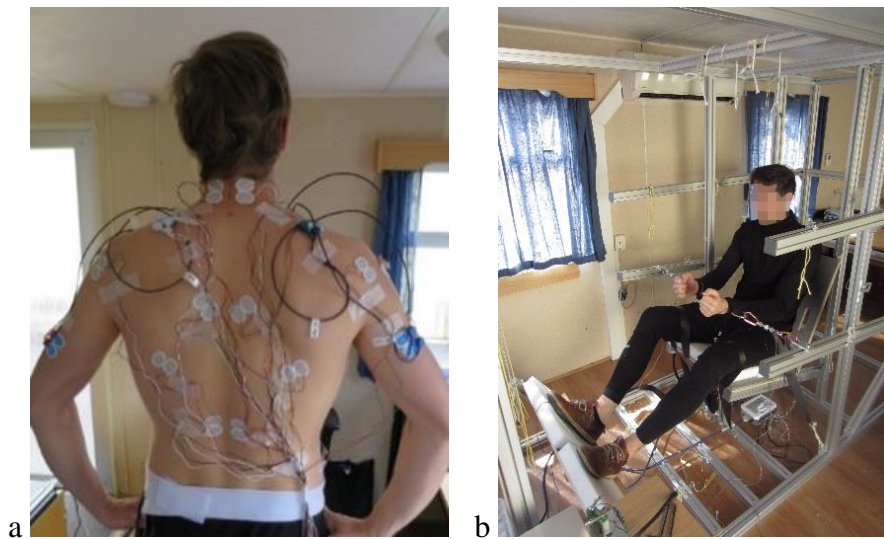
Fig. 7. EMG electrodes on a volunteer's upper body (a) MVC test rig with a volunteer (b).
