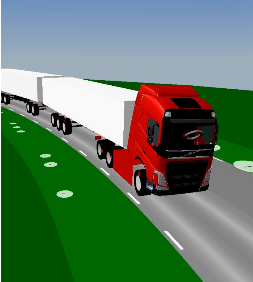
A-double motion, braking the dolly's 2nd axle (animations)
