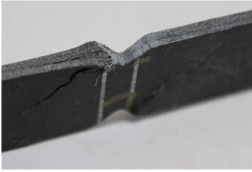
Figure 12. Edge crushing on tabless specimen.
