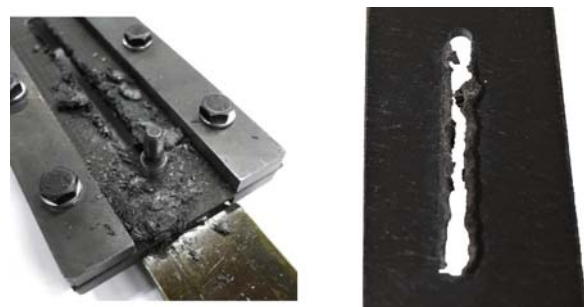
Figure 1. Post tearing test specimen [16] (left); a random fibre CF-PP specimen after tearing [17] (right).
