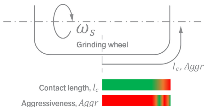
Fig. 21. Changes of aggressiveness and contact length across the profile of the grinding wheel in crankshaft grinding.
