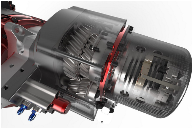
Fig. 6. Rimac Automobili's (Concept_One) high-speed dual permanent-magnet electric motor (600 kW peak power, 12,000 RPM) featuring a double-clutch two-speed gearbox [148].
