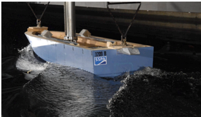
Fig. 1. The flow pattern around a planing transom stern hull at two different speeds. The hull transom is wet below the critical speed (left), and it becomes dry above the critical speed (right).
