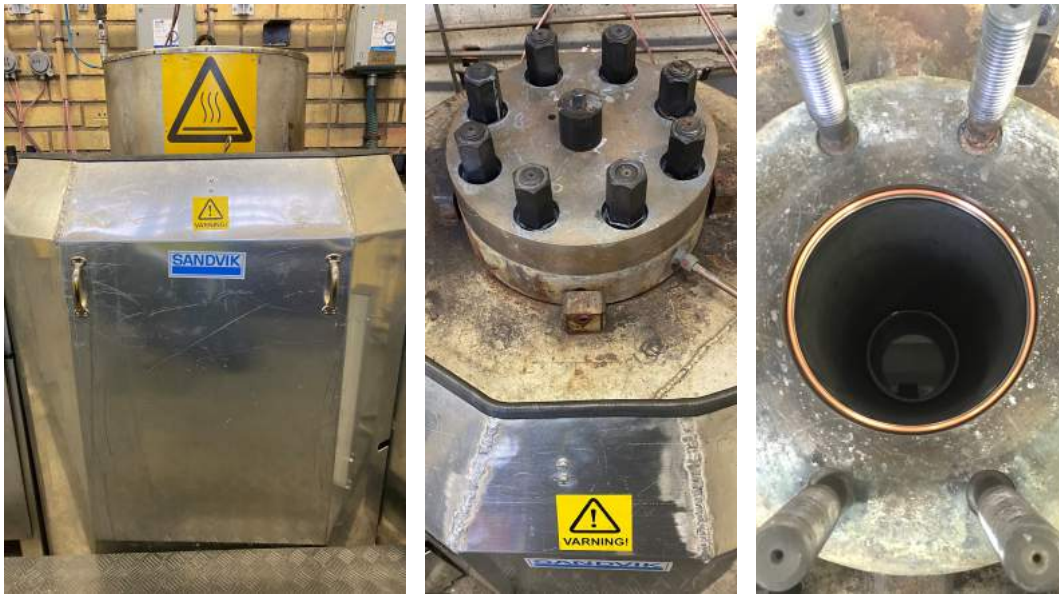
Figure 4-2: The autoclave setup: the autoclave (left), the top without cover (centre), the inside (right).
