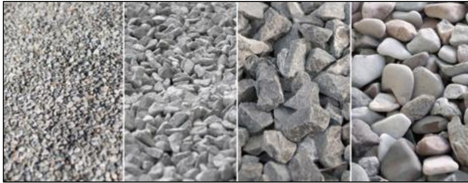
Figure 1. Photographs of 4 different types of rocks with varying levels of roundness and angularity.
