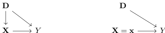
FIGURE 1. (left) Causal diagram described by \mathfrak{G} ; (right) causal diagram altered according to the intervention \mathbf{X} = \mathbf{x} .
