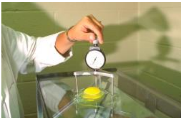
Figure 1.8. Demonstration of the use of a Haugh meter (USDA, 2000).
