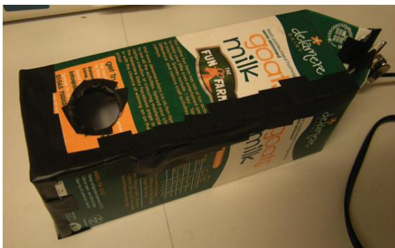
Figure 2.5. Homemade egg candler. Each egg was placed on the hole (left hand side of the box) and examined in a dark room with the cadler light switched on.
