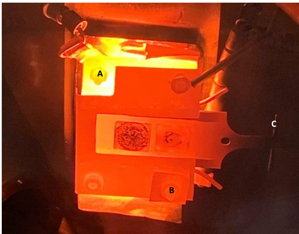
Figure 4.2.4: Boralectric heater annealing a sample at high temperature in the analysis chamber, with the cone of the analyser in the left corner. Current is passed through bolt A to B, where the bolts go through the heater and make contact with the PG centre. C labels the wings which lock the sample plate into the magnetic arm for transferring samples between chambers.
