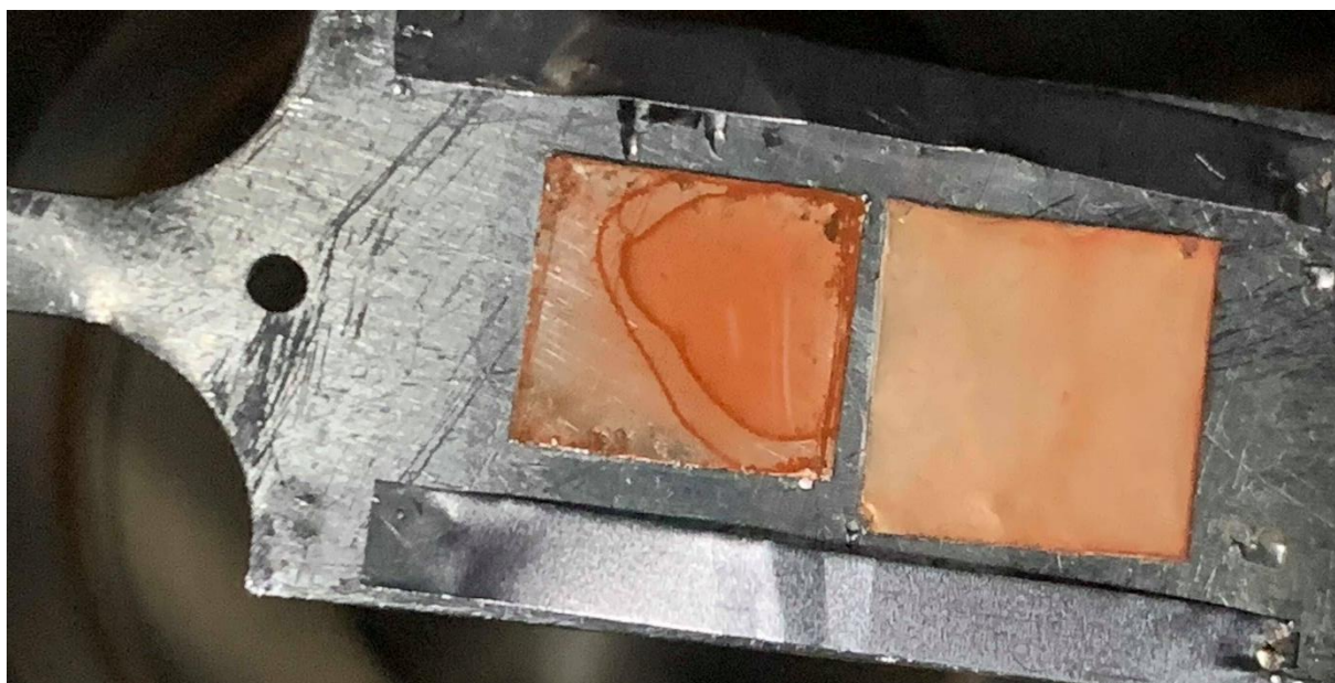
Figure 4.2.3: Image showing two hematite nanoparticle films which were created via drop-casting 3\mu\text{L} and 1\mu\text{L} respectively onto platinum films and then slowly pumping down the load lock to 5 \times 10^{-10} mbar and maintaining the pressure until all water has evaporated. The larger droplet formed coffee rings due to the 3\mu\text{L} droplet having a larger meniscus, and therefore parts of the droplet evaporating at different rates.
