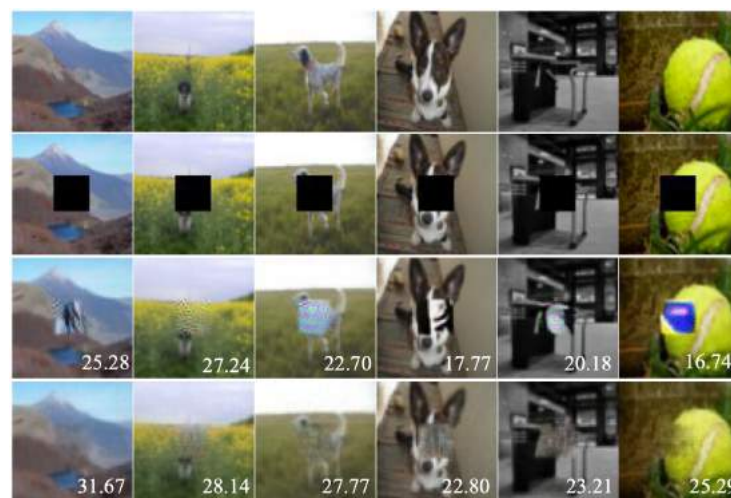
Figure 1. Examples of Blockwise Inpainting, where GAN based methods can be prone to overfitting but our network is not. Rows from top to bottom: original images; the masked input images; the outputs of OneNet [12] showing evidence of overfitting; the results of our network. The figures show the PSNR of the output images. We have reproduced the examples selected by the authors of [12] using their code [31]. The OneNet examples in [15] show similar problems for blockwise inpainting.
