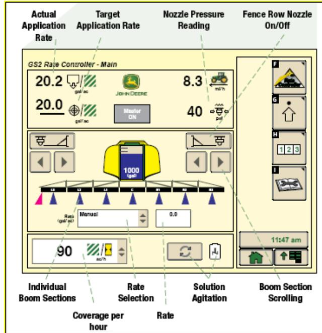
Figure 1. GreenStar 2 (GS2) Rate Controller screen shot taken from [http://www.deere.com/en\\_US/ProductCatalog/FR/literature/2009/ams/dsaa40430\\_all\\_greenstar\\_products.pdf](http://www.deere.com/en_US/ProductCatalog/FR/literature/2009/ams/dsaa40430_all_greenstar_products.pdf), p. 20.
