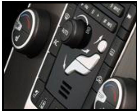
Figure 1. Analogous use of human anatomy in a Human-Machine Interface. (Source: Volvo Car Corporation)
