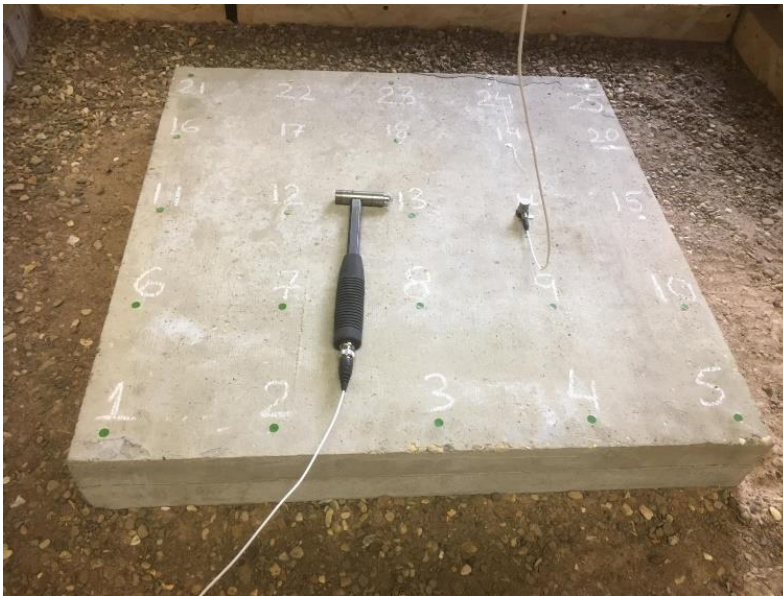
Figure 5-29: Test 05. Two slabs, 'full-debonded' supported on subgrade.
