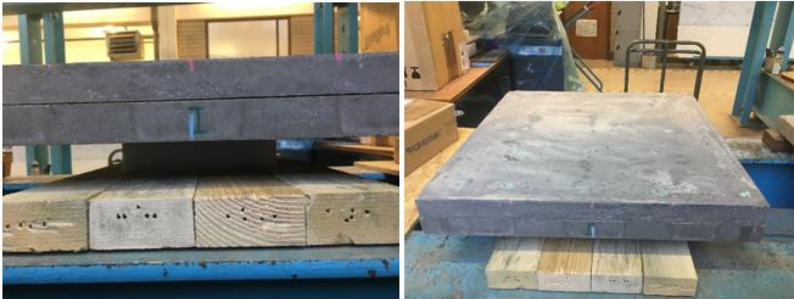
Figure 5-18: Test 02. Two slabs 'fully-debonded', supported on ETHAFOAM 220.
