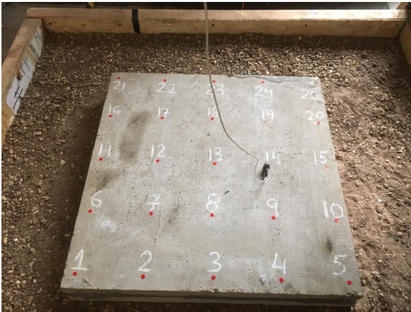
Figure 5-33: Test 07. Two slabs with '3 Delaminations' supported on Subgrade.
