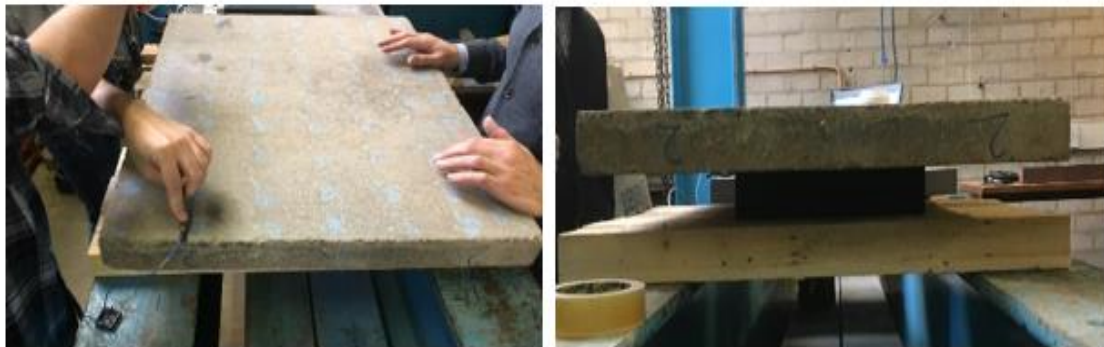
Figure 5-12: Test 01. Single 'robust' concrete slab, supported on ETHAFOAM 220.
