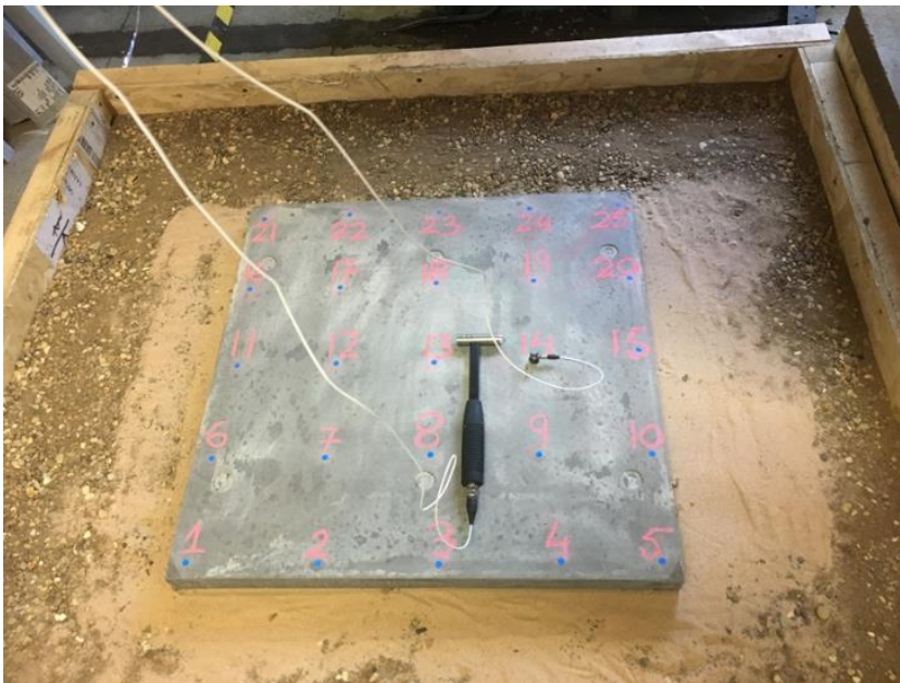
Figure 5-24: Test 03. Single ‘robust’ concrete slab, supported on subgrade.
