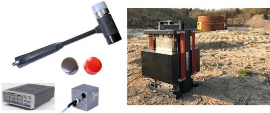
Figure 5-4: Impact Hammer, Piezoelectric triaxle accelerometer and Data logger. A Shaker, as an excitation source (PCB 2011).
