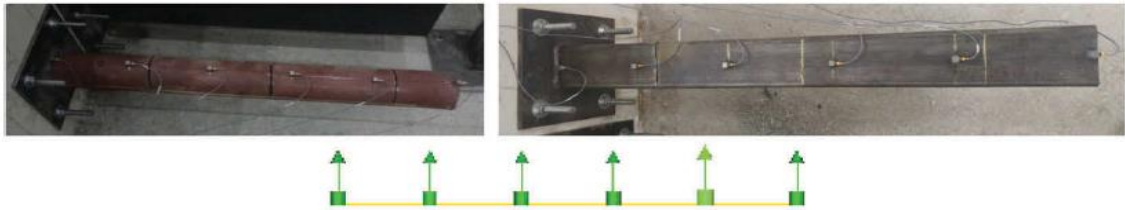
Figure 2-25: Lab scaled model of steel cantilever beams, mounted with accelerometers (Altunışık et al. 2019).
