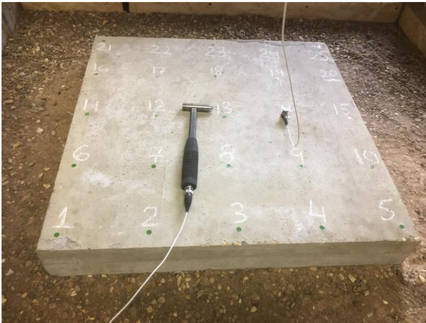
Figure 5-31: Test 06. Two slabs, 'fully-bonded' supported on subgrade.
